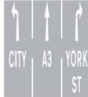
Indication of traffic lanes
